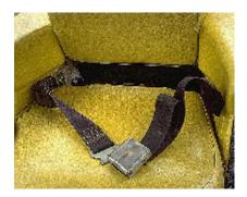
5. Seatbelt straps are properly anchored, and in excellent condition; straps and buckle are easily reached.
