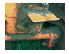
3. Master shield in place but a bend, crack or slice reduces its protection; original or current shield offers poor protection.
