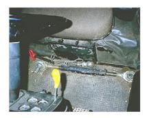
3. Operators platform is relatively clean, some tools are on platform but stowed out of the way of the operator. Most tools are in a tool box. The tool box may not be secure, is overfilled, or in poor condition.
