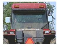
5. Mirror has all glass intact. An adjustable mirror is on each side.
