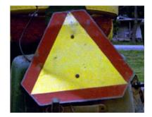
3. Faded, not in correct place; noticeably bent; upside down; partially obstructed; muddy.
