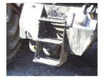
5. Good tread, clean, wide steps; operator's platform is no more than 27 inches high (steps are not required).
