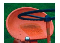
2. Seat twisted; cockeyed; no suspension; rusted-through seat.
